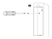
5. Screw back Positioning Screw into drill hole
