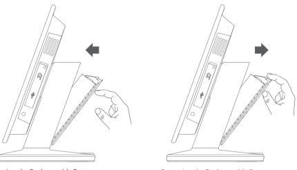
Placing the Rechargeable Battery
